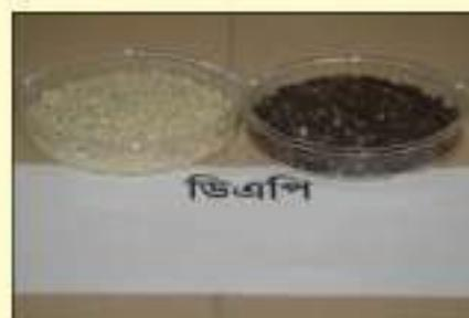
For quality testing, pour one teaspoonful of DAP into 100 ml of water in a beaker or glass. The good quality DAP will be dissolved quickly. After dissolution, add half teaspoonful of barium chloride ( $BaCl_2$ ) into the solution. In case of good quality DAP,  $BaCl_2$  will be settled down at the bottom of the beaker or glass. On the other hand, adulterated DAP will produce turbid/muddy/hazy precipitate in the solution due to presence of sulphur.
